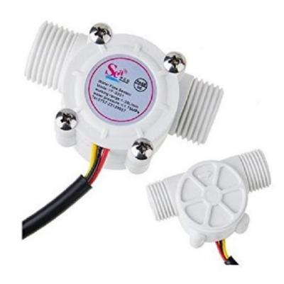
This sensor sits in line with your water line and contains a pinwheel sensor to measure how much liquid has moved through it. There's an integrated magnetic hall effect sensor that outputs an electrical pulse with every revolution. The hall effect sensor is sealed from the water pipe and allows the sensor to stay safe and dry.
